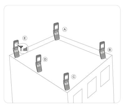
As shown from the above illustration, testing the signals from A to E, and select a best place that displays full bar Signals to install the donor antenna. Temporarily mount the Donor (outside) antenna in that location. It may need to adjust and move the antenna later.
