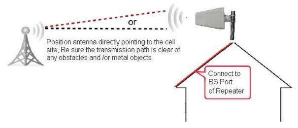
Find the location and best angle for getting the strongest signal from the base station. The antenna must be directed towards the nearest base station.
